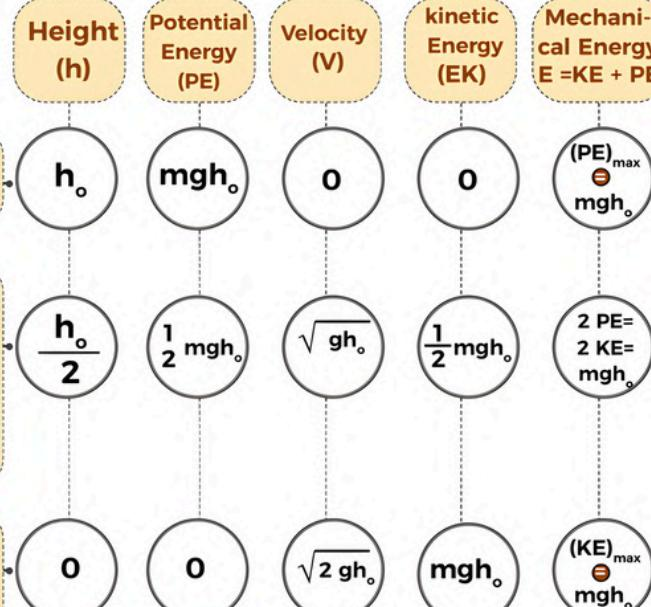
In the case of a simple pendulum oscillation, as shown in the figure:
